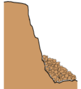
Eventually after repeated freezing and thawing, the rock breaks off.
